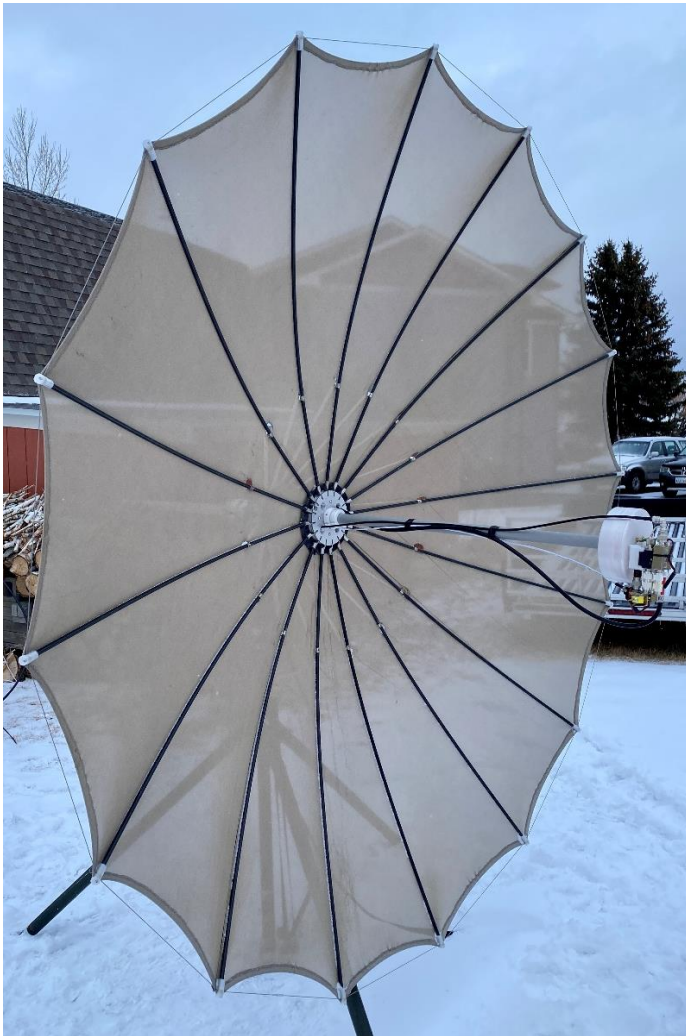
KB7Q 2.4 m portable folding dish with patch feed
