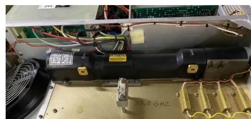
PA0EHG's 38 GHz 40W TWTA with WR22 output
