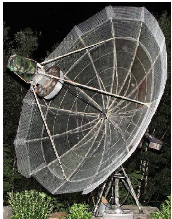
KA1GT's extended dish with 23 cm feed
