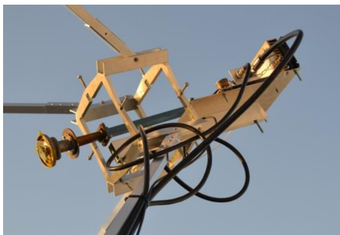
Miguel's 3 cm feed... The new system is working well with a Moon noise of ~ 1.3 dB.
