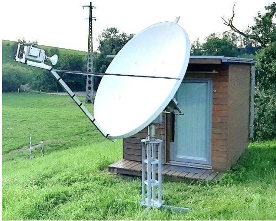
OK2QA EME QTH and 2.4 m offset dish
