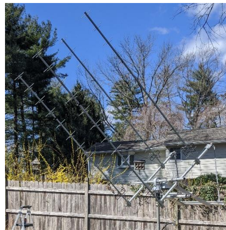
W2HRO's new 4 x cross yagi array for 432
