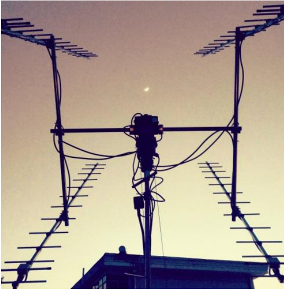
BD9BU 4 x 13 el DK7ZB yagis array used on 432
