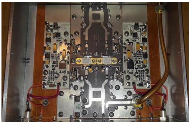
VE6BGT's 6 cm 100W PA (based on SM6PGP design)
