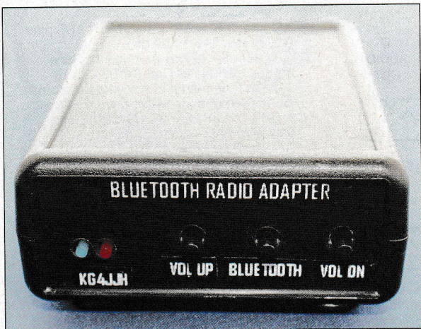
Figure 2 — Select the Bluetooth features using the three front panel pushbuttons and observe the Bluetooth state indications on the red and blue LEDs.
