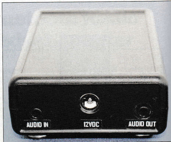
Figure 3 — Audio in and out, and 12 V dc connections are on the rear panel.
