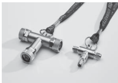
Figure 3-11. Convenient calibration components for the VNA provide the Open, Short and Load standards for the SOLT calibration procedure.
