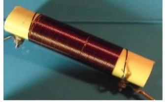
C1 = 150pf 2KV L1 = 2 x 7 turns + 2 turns bifilair on a ft140-43 L2 = 35uHwire 1 = +/-10.15m wire 2 = +/- 2.15m
