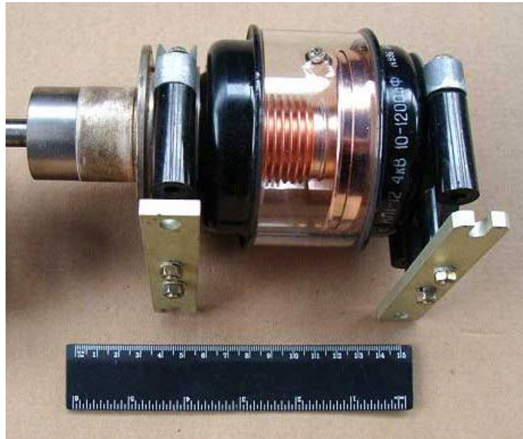
Figure 14 Russian Mil-style vacuum variable with integral clamps
