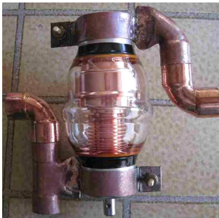
Figure 13 Homebrew capacitor clamps with silver-soldered copper fittings
