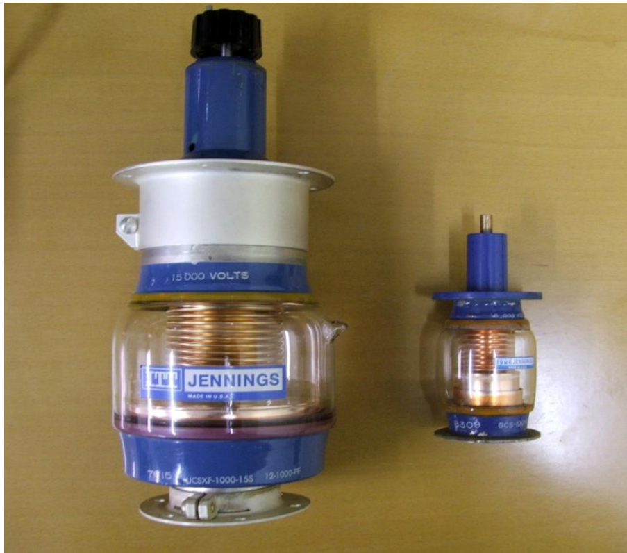
Figure 2 Vacuum variable style low-loss capacitors
