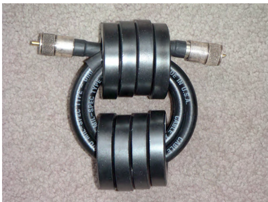
Figure 7 Multi-turn high power common-mode choke balun
