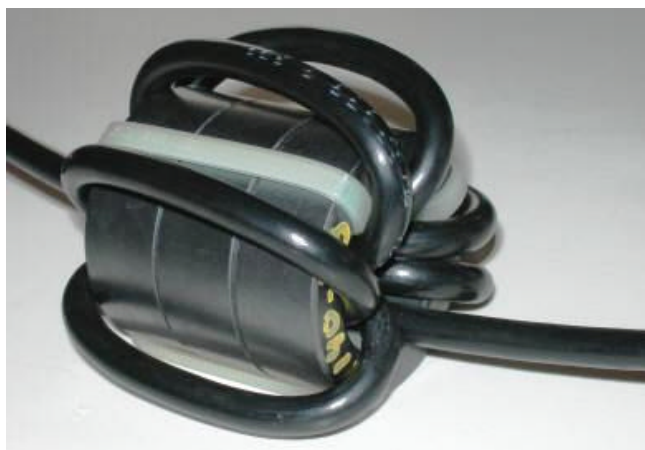
Figure 9 Alternative common-mode choke construction
