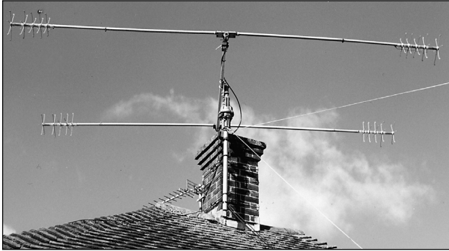
Fig 13.44: A compact two-element multiband beam
