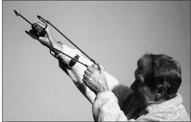
Fig 13.43: An antenna support catapult launch pad. The catapult is held nearly upside down so that the line does not get caught up with anything when fired. It is advisable to gain proficiency with few practice runs in an open space before using it to secure an antenna support.
