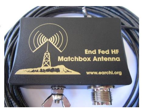
Best performance is achieved with a coax of 16' or longer with the coax shield providing the counterpoise function. Additional counterpoise is usually not required in this design, although the lower wing nut provides a convenient counterpoise connector if needed. The end fed antenna system works well in horizontal, sloper, and vertical configurations.
