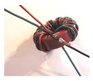
Trim and strip the remaining <u>right green</u> wire at about 2". Cut an additional 2" piece of green wire, and crimp and solder both wires to a # 8 lug. The 2" green wire will connect to the ground
