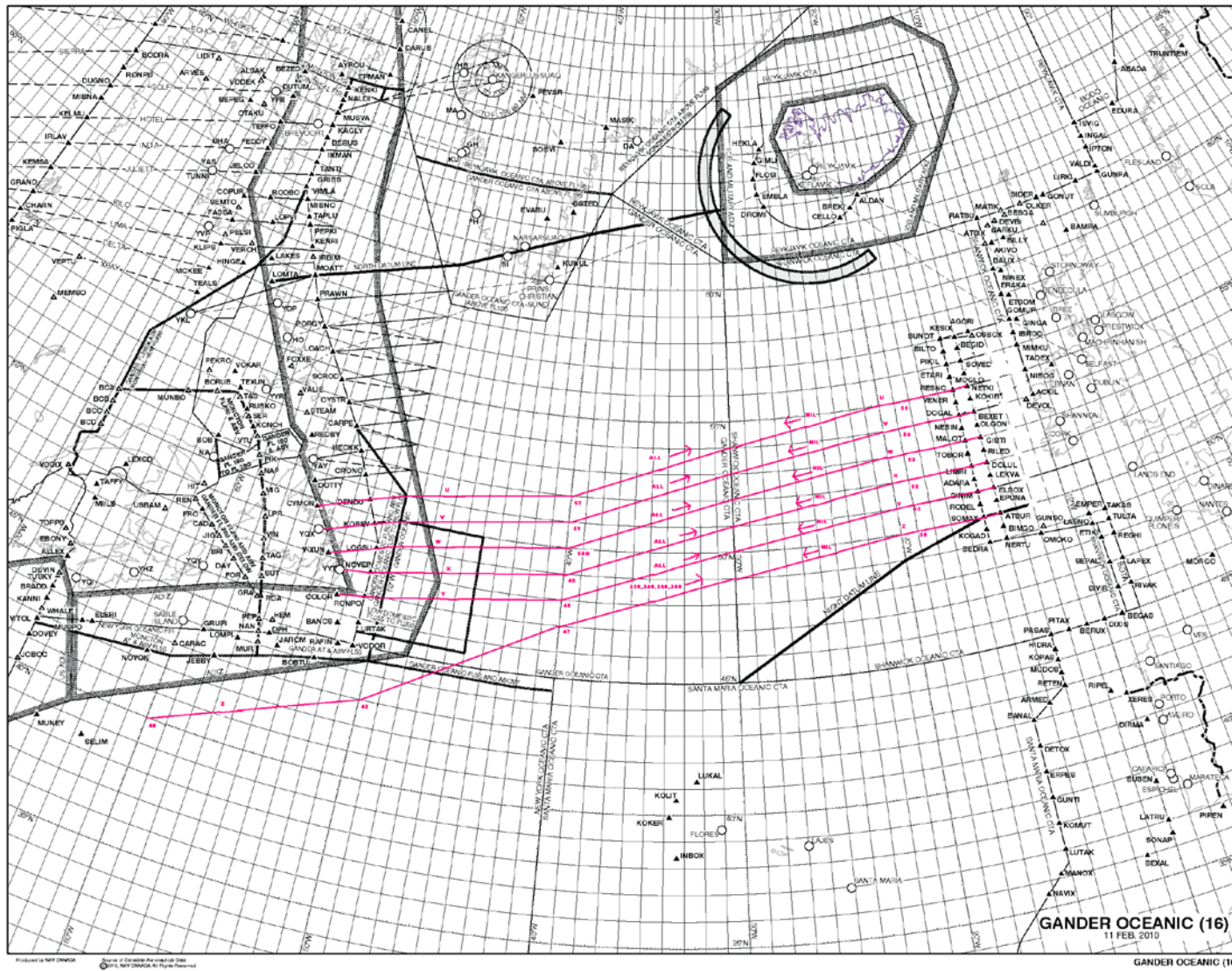
Figure 2 - - Example of Night-time Eastbound Organised Track System
