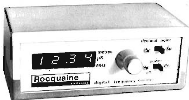
DFM from Roquaine Electronics operates up to 40MHz. It can be coupled to the receiver to provide direct readout of frequency. Unusually, wavelength can also be displayed
