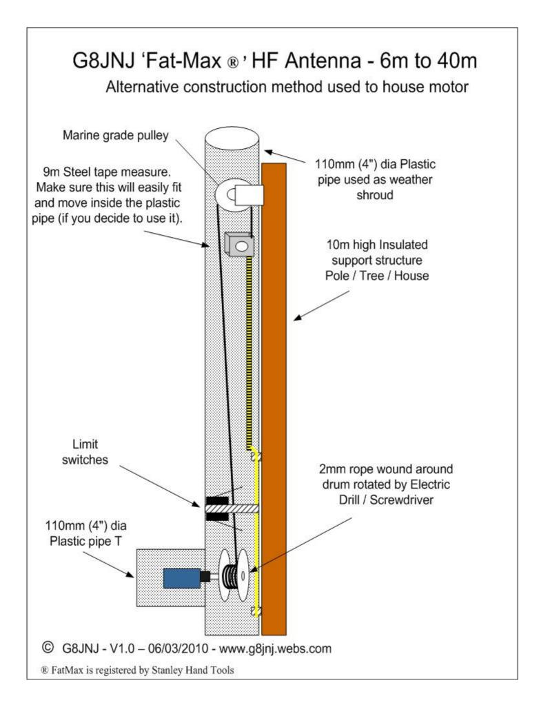
Installing the tape measure in a plastic pipe will reduce the length of tape required for the vertical element slightly, due to its dielectric loading properties. However it may be possible to either shorten the antenna, or make it resonant on
