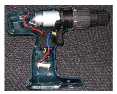
With a 12v Drill motor and 1" spindle the rate of cord movement was about 1m per second. At 5V it was about 0.5m per second.
