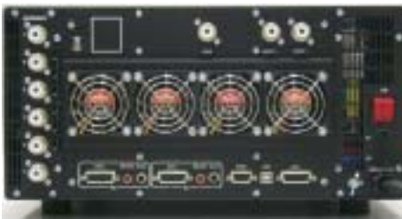
SPE 2K-FA rear panel showing six antenna outputs, two drive inputs and SO2R input.
