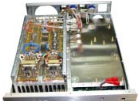
IØJXX Compact Vario internal view. Two separate RF amplifier boards and two sets of T/R relays are visible.
