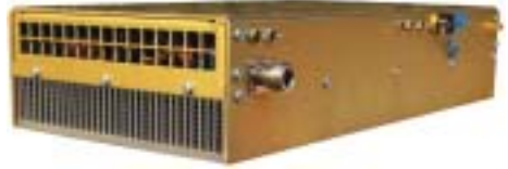
IØJXX 50MHz 1000 Watt Box Amplifier.
