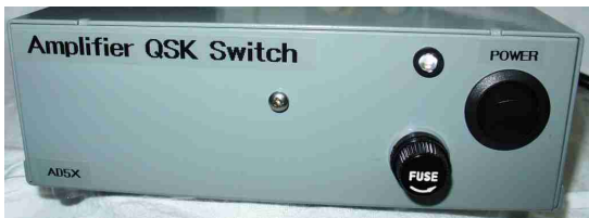
Photo E: Front View of the QSK Switch.
