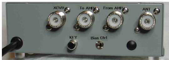
Photo F: Rear view of the QSK switch.
