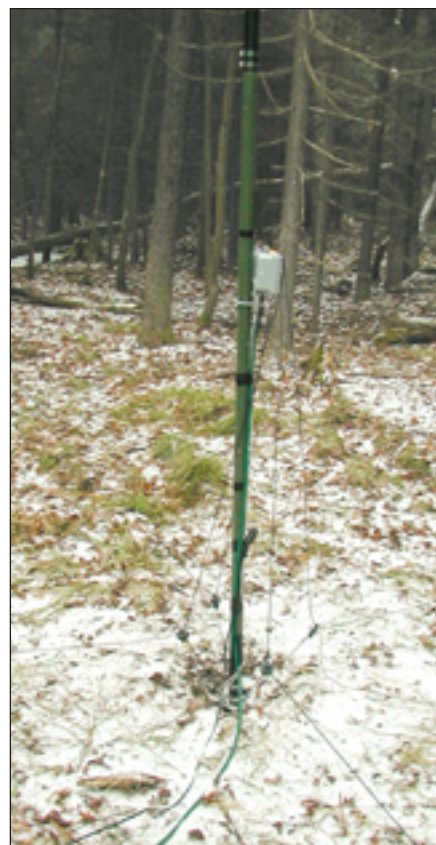
Figure 7 — The green fiberglass mast, black wire and black Dacron guy ropes all help the assembled AS-AYL-4 MW mast/wire kit blend into the background. The gray relay box is mounted several feet off the ground with the ends of the loop wires attached to posts on top.
