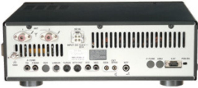
Figure 4 — The FT-950's rear panel includes connections for two antennas, a linear amplifier, and digital mode interface. Other jacks allow for plug-and-play connection to Yaesu optional \mu -Tune units, data management unit, FC-40 external antenna tuner and VL-1000 power amplifier.
