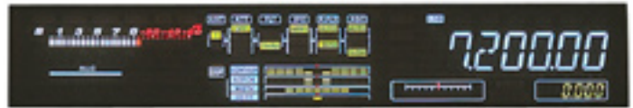
Figure 5 — As with other current Yaesu HF transceivers, the display shows filter selection, DSP settings and other important operating parameters at a glance.
