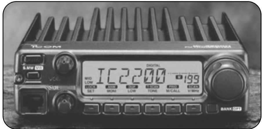
Photo A. The ICOM IC-2200H is a conventional 2-meter FM transceiver with D-STAR digital operation available as an option. (Photo courtesy of ICOM America)
